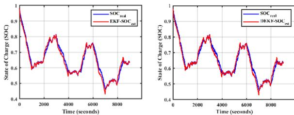
Fig.3 (a) EKF-SOC (b) DEKF-SOC with input current bias respectively
