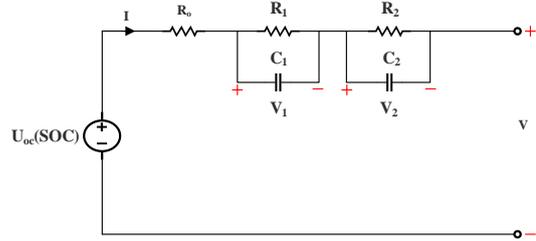
Fig. 1 Second-order battery equivalent circuit model
